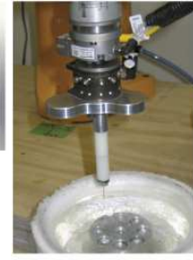
Figure 8-16 Robotic cryoquenching of a mounted crystal. The robot arm carries the crystal on a cryo-pin with a magnetic base and is about to dip it into the storage puck submerged in liquid nitrogen. Note how the liquid nitrogen is boiling, and that the crystal will travel through a cushion of cold nitrogen gas first before it is quenched into the liquid nitrogen itself. Blowing the gas cushion away with dry nitrogen drastically increases the quenching rates. 37 This robot is also a prototype capable of semi-automatically harvesting crystals, and autonomous crystal harvesting is a remaining frontier in full automation of high-throughput crystallography. 38
