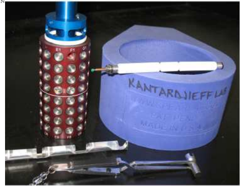
Figure 8-14 Various cryotools. The picture shows a variety of common tools used during cryomounting and cryostorage of protein crystals. The blue vessel is an unbreakable foam Dewar made by SpearLabs from closed cell foam. On top of it rests a magnetic wand used to hold and manipulate the mounting pins. A Hampton base with a copper pin is shown; stainless steel pins are more frequently used. The storage cylinder to the left of the foam vessel is an SSRIL design. It fits the bore of a shipping Dewar and the pins can be auto-mounted by the SSRIL beam line robotics. Below the cylinder is a simple aluminum cane that holds a series of cryo-vials with a magnetic rim securing and protecting the mounting pins. Several of these canes can be stored in a shipping or storage Dewar. At the bottom of the image is a cryo-tong that is pre-cooled under LN 2 and used to transfer pins from storage or quenching vessels onto the diffractometer. Tools and samples are kept at cryogenic temperatures at all times during mounting.
