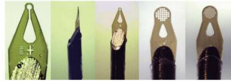
Figure 8-13 Harvesting and flash-cooling process. The crystal is scooped up from the drop in a mounting loop on a pin, and dipped quickly into liquid nitrogen. A vial with a magnetic rim placed in a submerged storage puck protects the mounting pin. The insert shows a harvested crystal in an old-style hair (cat-whisker) loop.
