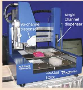
Figure 3-33 A robot for automated crystallization plate setup. The Phoenix robot (Art Robbins Instruments) can set up 96 crystallization trials in about one minute. On the left side, a 96-channel syringe dispenser re-arrays (100 \mu\text{l} each) 96 prefabricated or purchased crystallization cocktails simultaneously from a standard deep-well block into the reservoirs of an SBS-format, 96-well sitting-drop crystallization plate, and places between 1 \mu\text{l} and 100 \text{nl} into the drop shelves or wells. From the right side, a contact-less microvalve dispenser nozzle immediately adds the pre-aspirated protein (stock vials in the red block) rapidly and without contact onto each of the precipitant drops. To minimize evaporation, the plate is then immediately sealed with a sheet of pressure-sensitive adhesive. Taking all losses into account, about 12 to 15 \mu\text{l} of protein stock is required for 96 100 + 100 \text{ nl} drops. The robot design has been based on a prototype developed in an academic laboratory setting. 44
