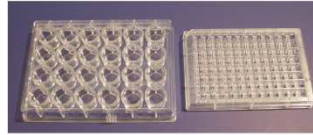
Figure 3-2 Crystallization plates. A 24-well Lindero plate used for a manual hanging-drop crystallization setup is shown to the left. Originally designed for cell culture work, the Lindero plates made from polystyrene are cheap and commercially available with pre-greased rims. The wells are covered with siliconized 22 mm circular cover slides. Although not suitable for automated work, the hanging-drop method using Lindero plates is still useful in small laboratories. The crystallization plate to the right is a typical 96-well sitting-drop plate in the smaller, standardized high-throughput SBS (Society for Biomedical Sciences) format (tradename, Art Robbins Instruments). Crystallization robotics most frequently use sitting-drop plates with a SBS footprint.
